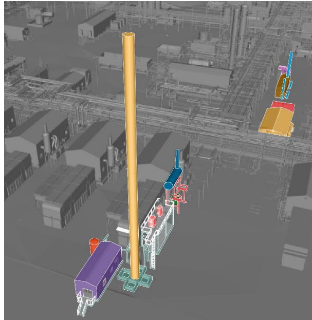
Absorber tower for one compressor engine
